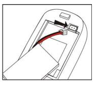
**b^{\times}** will be shown on the LCD screen if the battery has been properly connected. In the case **b^{\times}** is not shown, please check battery connection or charge the battery.
